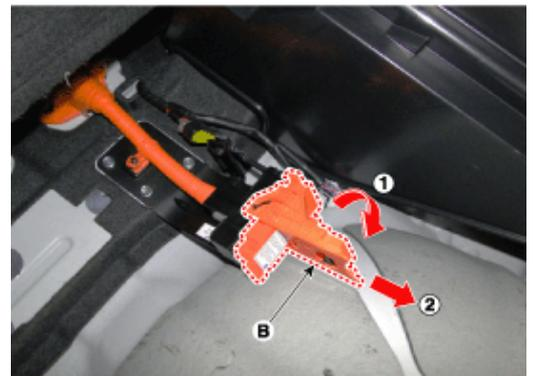
If neither of the preceding methods can be completed, emergency responders must be aware of the potential for accidental SRS activation as well as understand that there is no guarantee that the high-voltage system has been shut down.
