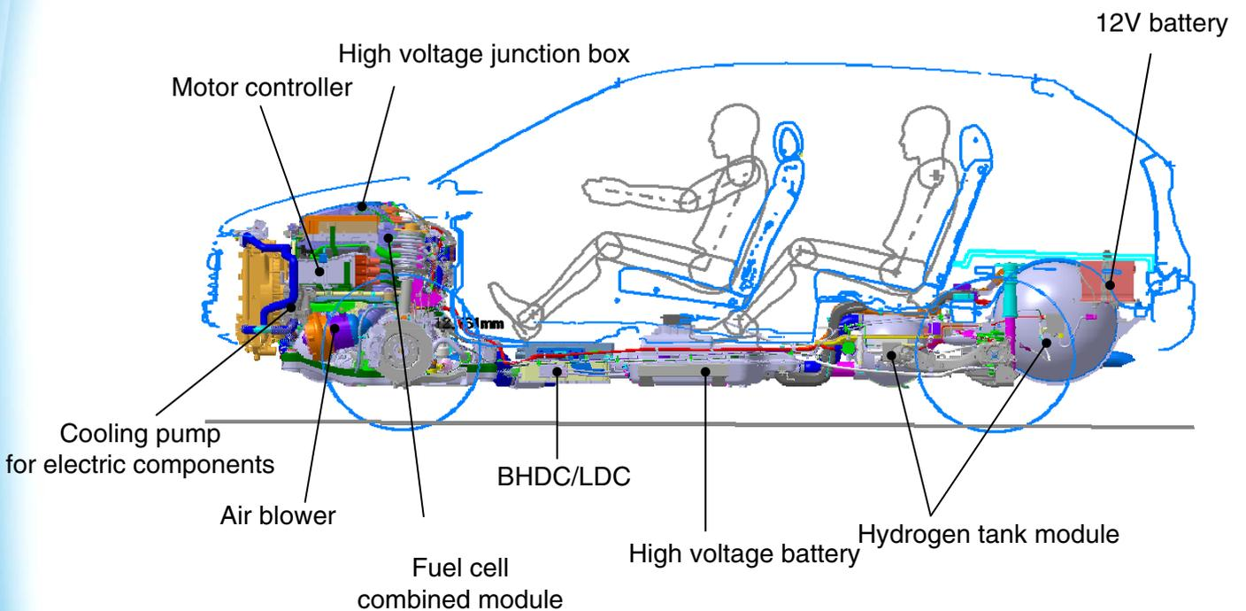
※ BHDC : Bidirectional High voltage DC-DC Converter
