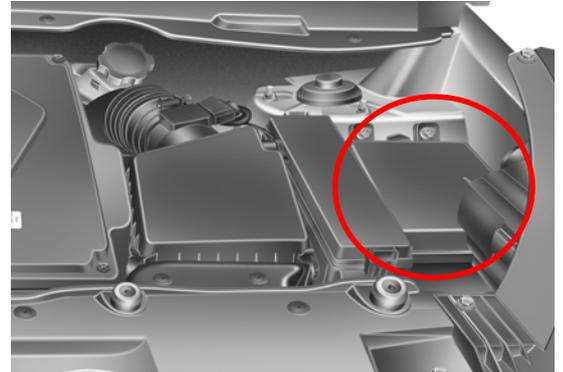
3. Remove the IG1, IG2 fuses. Refer to the illustration for fuse location.
