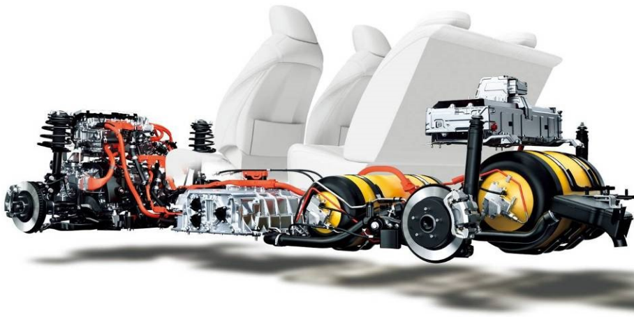
Figure 5 Example of a fuel cell powertrain (Source Toyota)
