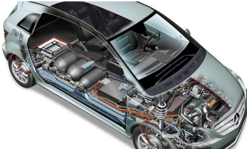
Figure 4 Example of a fuel cell powertrain (source Mercedes via EDUCAM)
