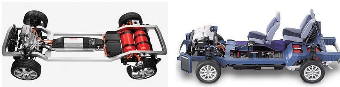
Figure 2 Design of a fuel cell chassis (source Honda).
